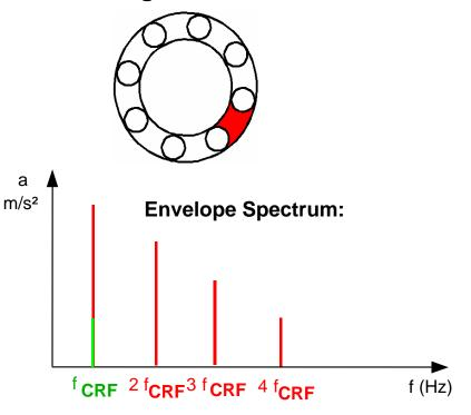
Cage rotational frequency  $\mathbf{f}_{\mbox{CRF}}$  and harmonics visible
